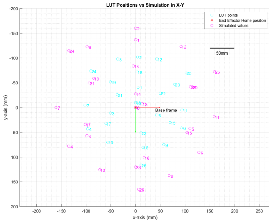
Robot Position Measurement vs Simulation Results in X-Y
