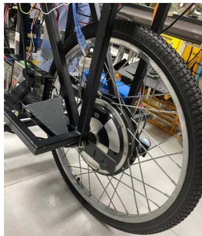
The Rear Wheel of a Self-balancing Bicycle
