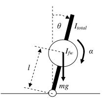
(b) If a PID controller is applied to control the system as shown in the below block diagram. Determine the closed loop transfer function and the ranges of the proportional, integral, and derivative gains that make the system become stable.
