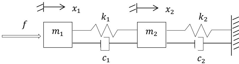
(a) Derive that the transfer function from the external force,  $f$ , to displacement of the second mass,  $x_2$ , is
