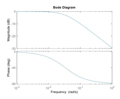
Characteristic equation of the desired time constant of 5 seconds 5s + 1 = 0 or s + 0.2 = 0. Characteristic equation of the system with proportional controller 30s + 1 + K = 0 or s + 1/30 + K/30 = 0
