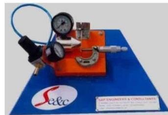
Figure 3.1.11-1 Nozzle-Flapper Transducer
