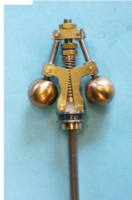
Figure 3.2.3-1 Flyball Velocity Pickup
