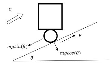
Since there is no slip, the friction force, F, will be the same as the tangential force from gravity,
