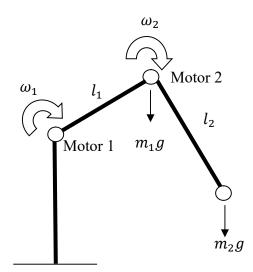
(a) When link 1 of length  $l_1$  is rotating at a constant speed of  $\omega_1$  and link 2 of length  $l_2$  is rotating at a constant speed of  $\omega_2$  and the links are considered as point masses as shown in the figure, determine the required power of both motor 1 and motor 2. Assume there is no safety factor is considered. (15)
