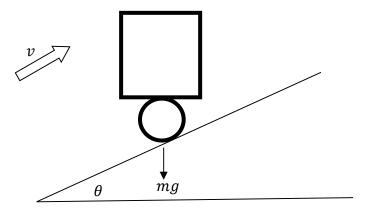
(a) When the robot has a total mass of m is running at a constant speed of v on a hill of slope  $\theta$ . The static friction coefficient between the wheel and the hill surface is considered very large and makes no slip, determine the required power from each wheel motor. Assume there is no safety factor is considered. (15)
