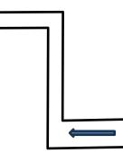
If the diameter of the pipe in the first floor is 2.5 cm and the diameter of the pipe in the second floor is 2 cm and the second floor is 3 m higher than the first floor. The flow is assumed frictionless and incompressible. Determine the flow rate if the pressure on the first floor is higher than the pressure on the second floor 30,000 Pa. Water has mass density of 1,000 kg/m<sup>3</sup> and gravitational acceleration is 9.8 m/s<sup>2</sup>. (20)
