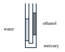
If both ends of the monometer are exposed to atmospheric pressure, determine the height difference between both ends of the manometer. Water, ethanol and mercury have the mass density of 1,000, 790 and 13,550 kg/m<sup>3</sup> respectively. (20)
