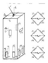
When the force with  $F_x = 20$  N,  $F_y = 10$  N,  $F_z = 30$  N, is applied, the voltage outputs from X, Y, and Z-Wheatstone bridge circuits are measured as 0.5 V, 1.2 V, and 2.4 V respectively. Determine the magnitude of an unknown force when the voltage outputs from X, Y, and Z-Wheatstone bridge circuits are measured as -1 V, 3 V, and -4 V respectively. (25)
