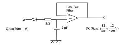
Select a low-pass first-order filter with cut-off frequency (3db attennuation) at 500 rad/s.
