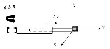
If the seismic mass deflects 1 mm from the acceleration of 10 m/s<sup>2</sup> in each axis, determine the deflections of seismic mass in all axes of the accelerometer at the instance when the first joint of the robotics arm is rotating at the angular position,  $\theta$ , of 0 rad, the angular velocity,  $\dot{\theta}$ , of 3 rad/s and at the angular acceleration,  $\ddot{\theta}$ , of 1 rad/s<sup>2</sup> and the second joint is extending and the
