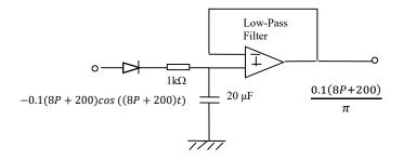
Select a low-pass first-order filter with cut-off frequency (3db attennuation) at 50 rad/s.
