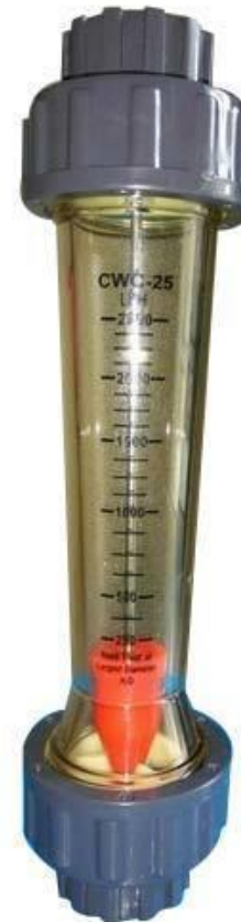
Figure 6.2.3.1-1 Rotameter (a) Principle of Operation (b) Glass-Tube Rotameter
