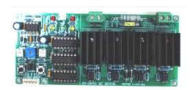
In the current setup, the board has limited applications for the DC motor, with a maximum draw of 10 amps. However, the proposed research introduces the use of
