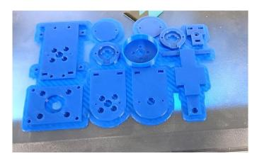
All the CAD designs of the unicycle robot were 3D printed using PLA material. Special care is recommended to print the 3D models. for this thesis, the CAD model is designed in such a way that it is 3D printable. All the settings for 3D printing are done using the fine option, with a shell thickness of 1.15 of nozzle size of 0.4mm.
