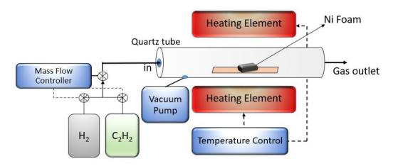
*Note.* Ni Foam was placed inside the quartz tube then being heated upto 700 C at 1 Torr pressure, C<sub>2</sub>H<sub>2</sub> is flow through the tube as precursor for carbon atom deposition. Very
