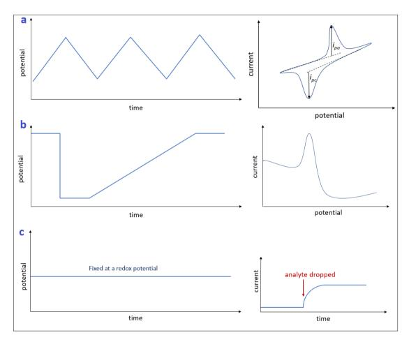
*Note*: (a) Cyclic Voltammetry (b) Anodic Stripping Voltammetry and (c) Chronoamperometry.
