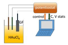
Most of electrochemical setup compose of three electrodes: (i) working electrode – where potential will be applied and reaction occurs, (ii) reference electrode – acting as a ground potential compared to working electrode potential and (iii) counter electrode – to complete electrical circuits.
